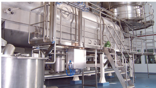
Spray Dryer and fluid bed dryer for instant whole milk
